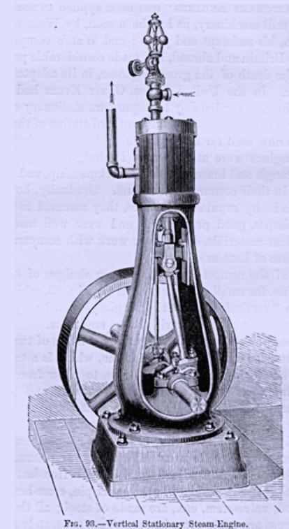
FIG. 98.—Vertical Stationary Steam Engine.
