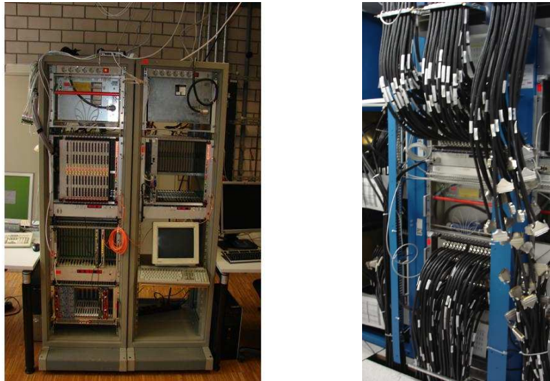
Figure 2.6: The full-crate test set-up built in the ATLAS Lab@KIP to test the PPMs (a) and details of the installation of the PPr System at CERN, in the electronics cavern of the experiment - as of August 2007 (b).
